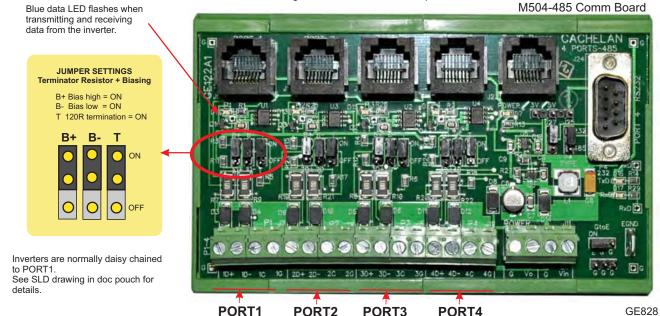
PORT1 PORT2 PORT3 PORT4 485 serial communication ports
